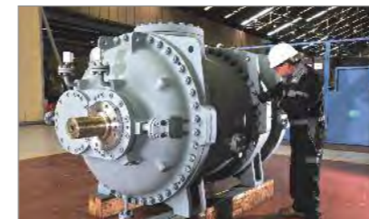
Above images show Howden rotary twin screw compressors designed and manufactured at Howden Compressors' global centre of excellence facility in Glasgow, Scotland, UK.
