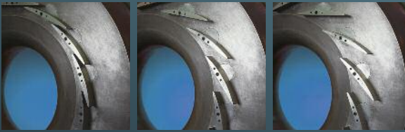
A. VVD closed B. VVD partially open C. VVD fully open
